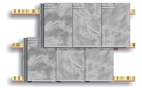
Tiles must be laid broken-bond and mechanically fixed according to specifications
